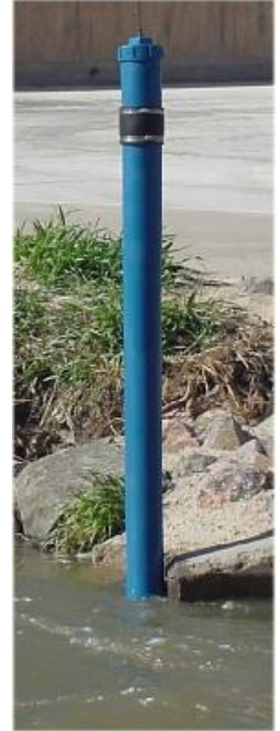
LEVELESE Wireless Sensor & Stilling Well in Creek
